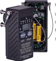
WilliamRDM's DVD is designed to withstand harsh environmental conditions and a drop from heights up to seven feet. It has a simple push-button design, which makes it easy to hold and operate with one hand, even when used with gloves.
